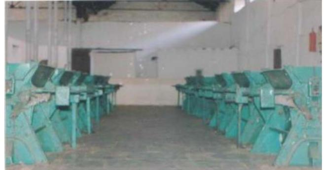
**Figure 3:** Battery of double roller (DR) ginning machines in a cotton roller ginning industry equipped with traditional chrome composite leather-clad rollers.
