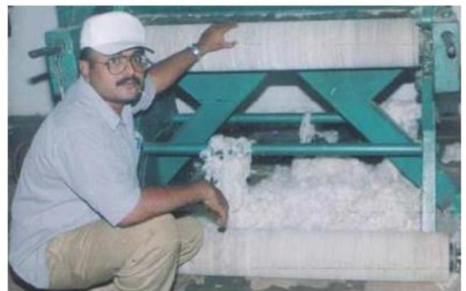
**Figure 8:** Gin rollers of double roller gin are made of rubberized cotton fabric roller covering material; green design-cast study-DPR-I.
